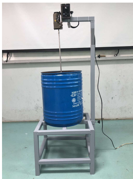
Figure 5. Prototype of a foam grinder with a waterproof flooring sheet molding from agricultural waste.
