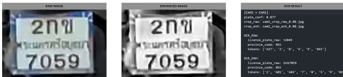
Figure 10. RAW vs Enhanced OCR Results
