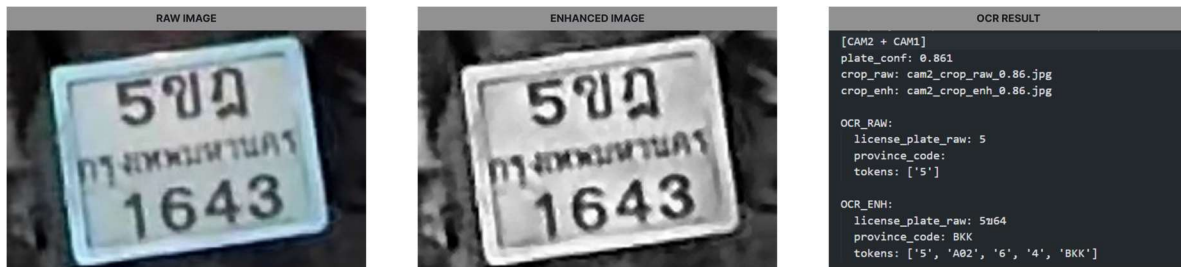
Figure 11. OCR Failure Cases
